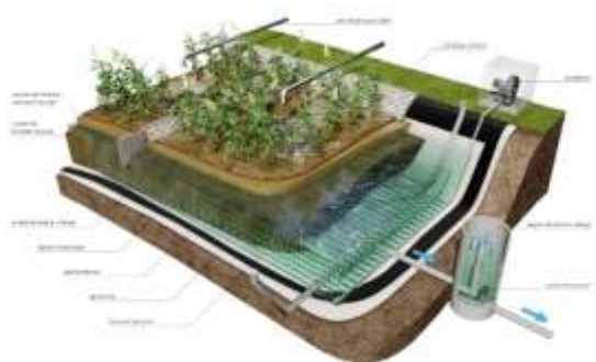
Figure 16. Diagram of effluent treatment by forced aeration Rhizosph'air®)
