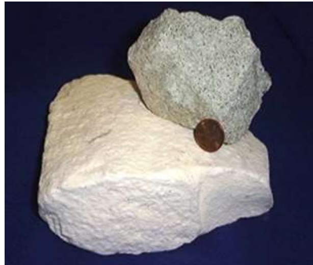
Figure 13. A zeolite is a rock formed by a microporous skeleton of aluminosilicate, whose voids optimize the adsorption and biodegradation processes of the reed root system. (Source Zeofito®).
